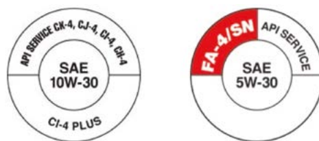
Figure 3. API symbols for CK-4 and FA-4 diesel engine oil categories. Clear distinction between CK-4 and FA-4 is necessary to avoid miss-filling the engines with not intended oils.
