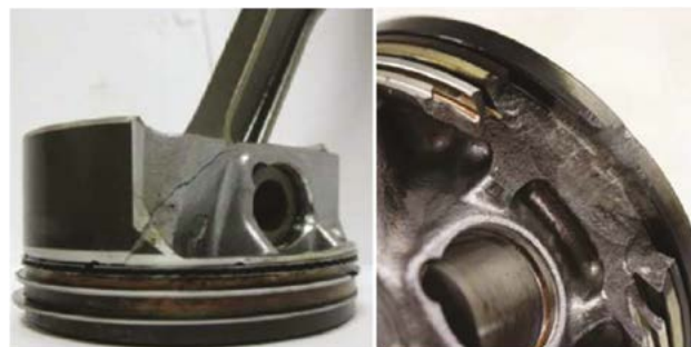
Figure 1. Two examples of piston damage due to LSPI.
